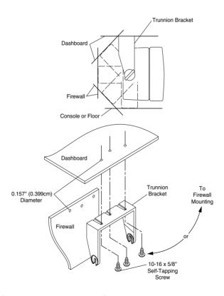
Figure 1-7 Mounting the Speaker Under the Dashboard
