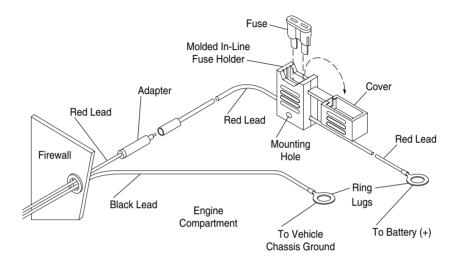
Figure 1-2 Power Cable Assembly
