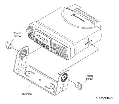
Figure 1-3 Radio into Trunnion
