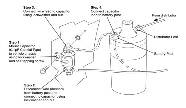
Figure 2-5 Ignition Coil Noise Suppression
