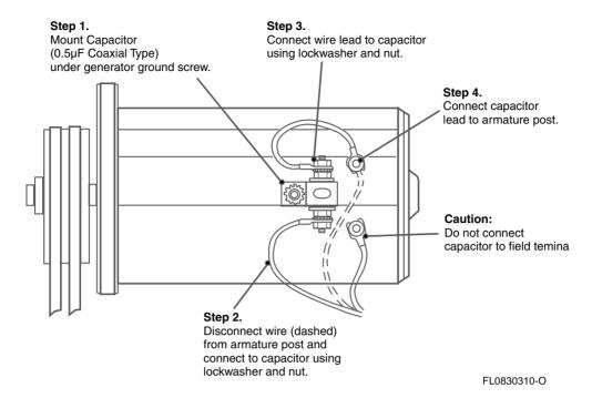
Figure 2-6 Generator Whine Suppression
