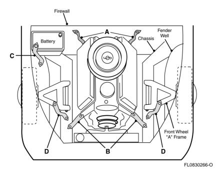
Figure 2-9 Ground Bonding
