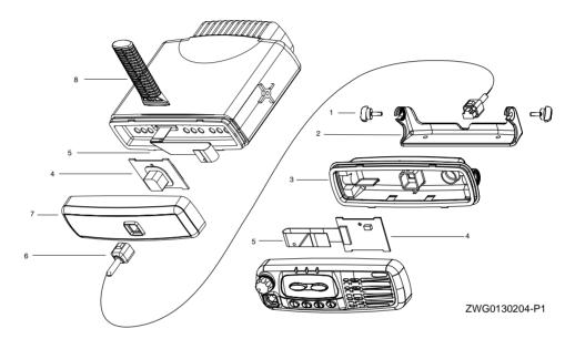
Figure 1-8 Remote Front and Back Housings
