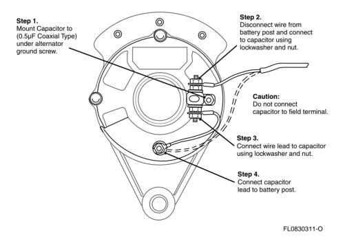
Figure 2-7 Alternator Whine Suppression
