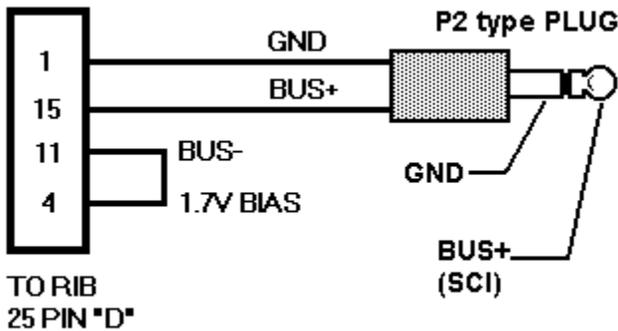
The programming cable is used for aligning the radio with the Motorola Radio Service Software (RSS). The RSS has NO other function than to service the radio, it is not for programming modes, editing repeater offsets, changing the scan list, changing frequencies, etc.
