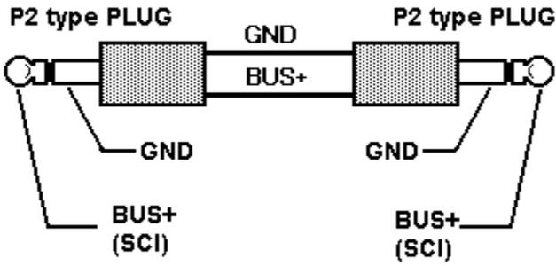
**Programming Cable Pinout**
